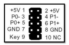
Figure 3: USB 10 pins Host male connector
