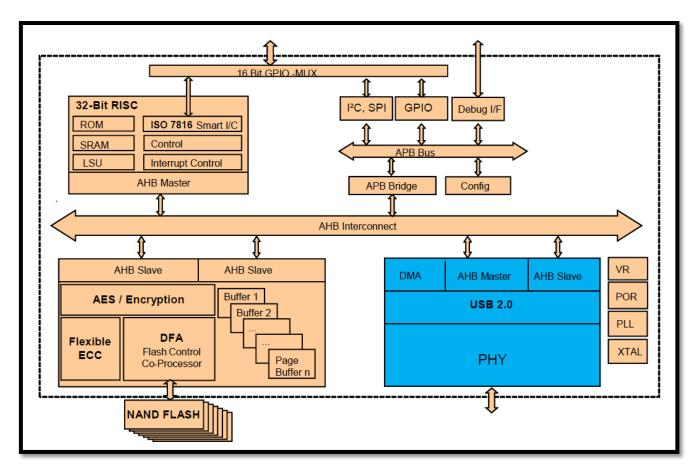
Figure 1: APRO SLC Micro USB Module (MUM) HERMIT-C Series block diagram
